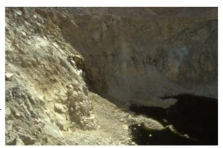
Open pit and underground mining operations are commonly excavating rocks below the natural water table. This will result in a drawdown of the water table, which can affect the water resources. Understanding the groundwater flow system and its connection to the surface water is essential. This class is designed for regulators and mining companies that will be dealing with mine-water hydrogeology.
